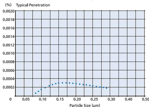
Esco cabinets use ULPA filters (per IEST-RP-CC001.3) instead of conventional HEPA filters commonly found in biological safety cabinets. While HEPA filters offer 99.99% typical efficiency at 0.3 micron level, ULPA filters provide >99.999% typical efficiency for particle sizes of 0.1 to 0.3 micron level.
